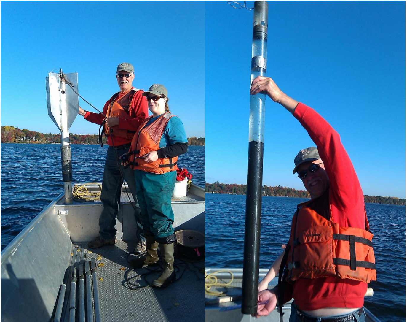
Paul Garrison and Gina LaLiberte with the DNR gravity corer about to drop into Red Lake's deepest area.
